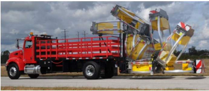
Truck-Mounted Attenuator (TMA) Most common, "folds up" during transport
